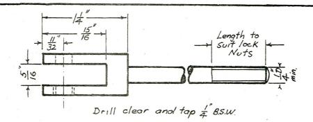
\* L to suit Drag Beam thickness, suitable compression spring, washer, Lock nuts plus approx ½ "of travel when spring fully compressed under load
